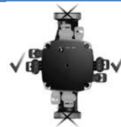
Control box position
