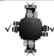
Control box position
